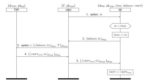
Fig. 3. Update protocol (typeset using the MSC package [10]).
