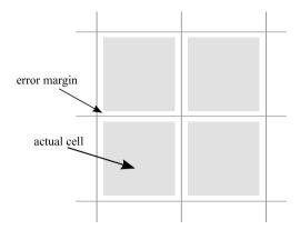
Fig. 2. Positioning system error margin around cells.
