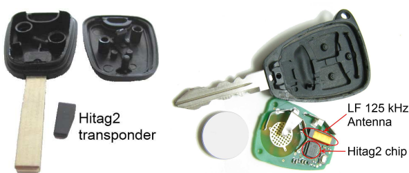
Fig. 1: Car keys with a Hitag2 transponder/chip
