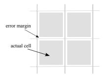
Fig. 2. Positioning system error margin around cells
